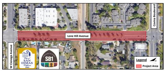
Project improvements include replacement of dilapidated cross gutter, sidewalk repairs and installation of new accessible corner ramps, as well as rehabilitation of the asphalt pavement section that will provide an aesthetically pleasing, smoother and quieter street surface lasting for many years.
